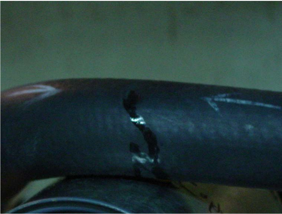
Close up showing hole in rad hose.
