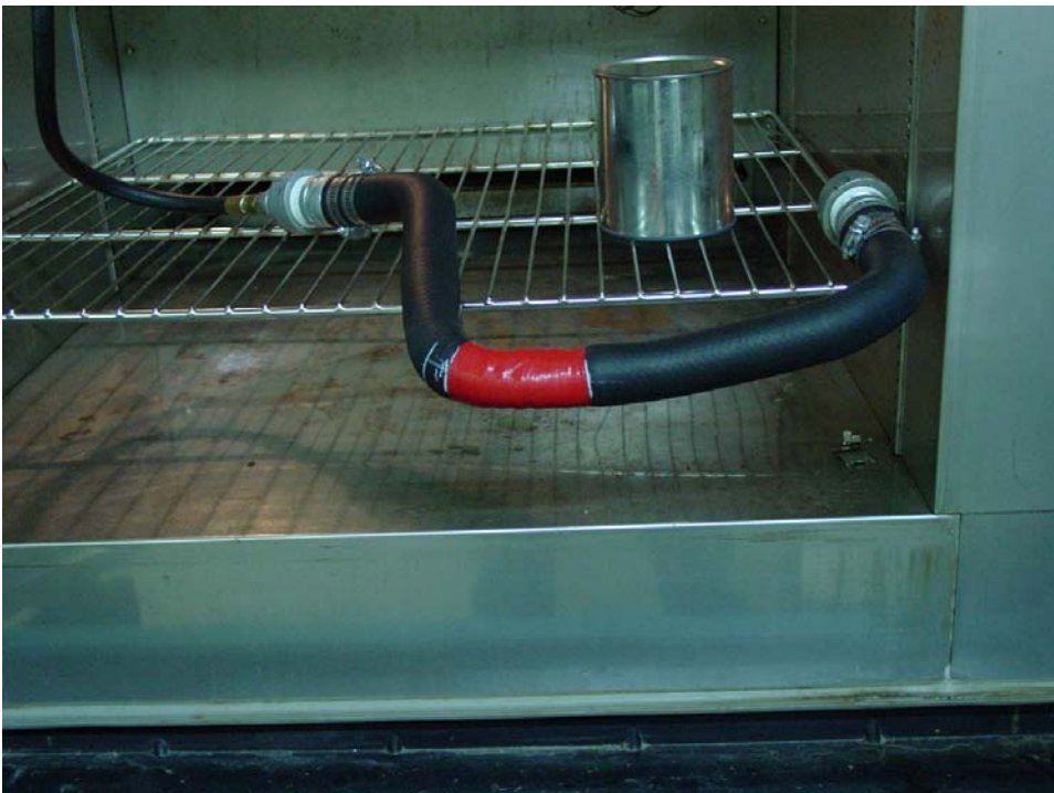
“Failure” repaired by tape under test.
